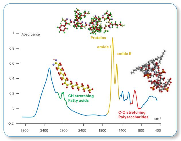
By default, the IR Biotyper analyzes IR spectra in the wavenumber range typical for carbohydrates (red), but other regions such as those indicating fatty acids (green) and proteins (yellow) can easily be selected for analysis in the software as well.
