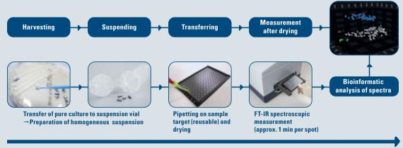
Using the IR Biotyper workflow, an entire batch of about 30 isolates (each with three replicates), plus standards, can be harvested, prepared and analyzed in about 3 hours.
